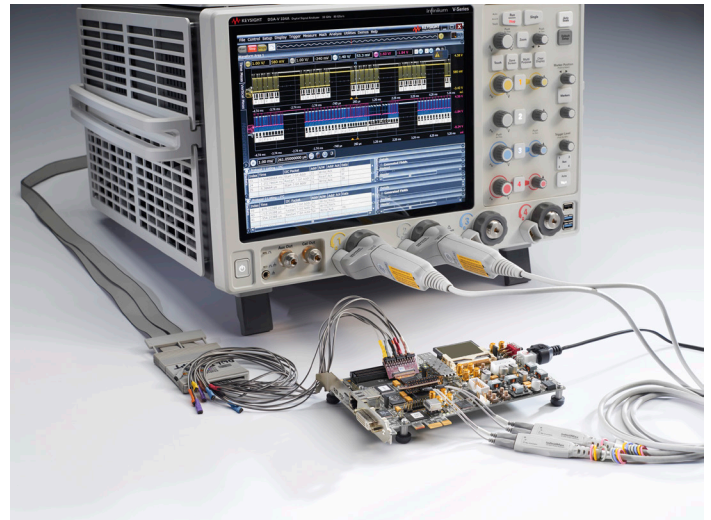
DDR3 test setup with mixed signal oscilloscope.
