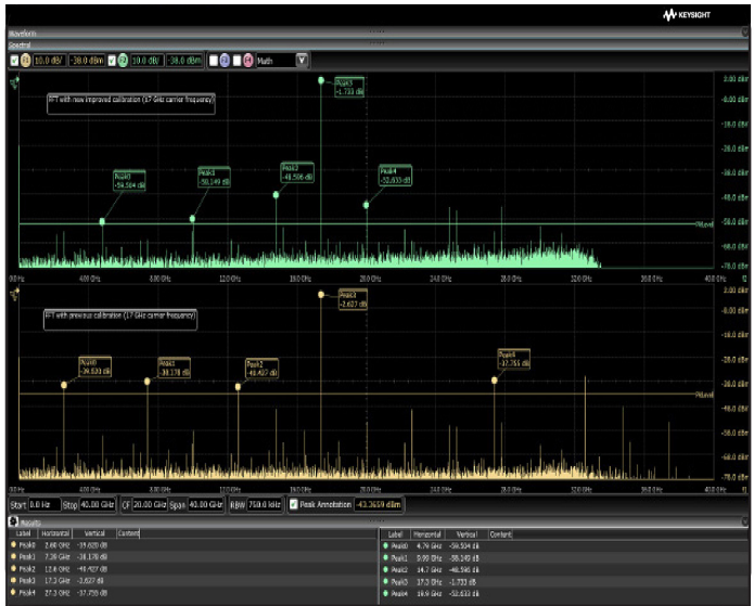
Improved calibration increases the spurious free dynamic range by up to 15 dBc.
