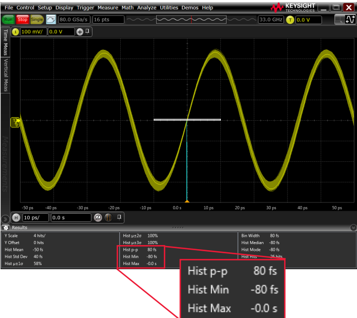
Jitter measurement floor of less than 100 fs (80 fs with 30 GHz input sine wave).
