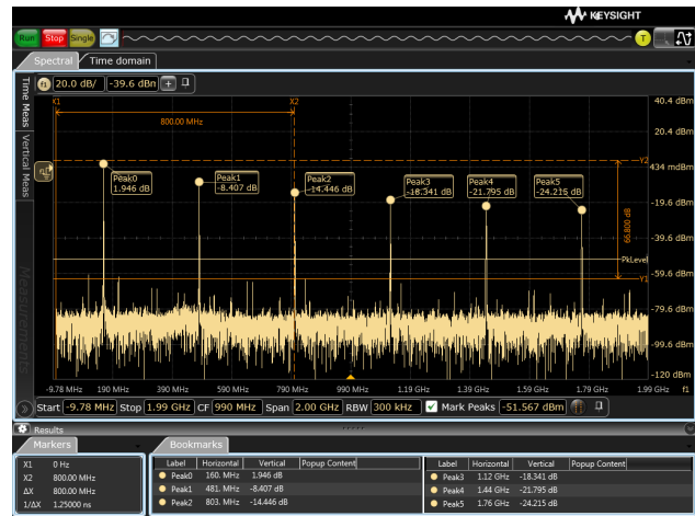
Peak readouts in the FFT plot.
