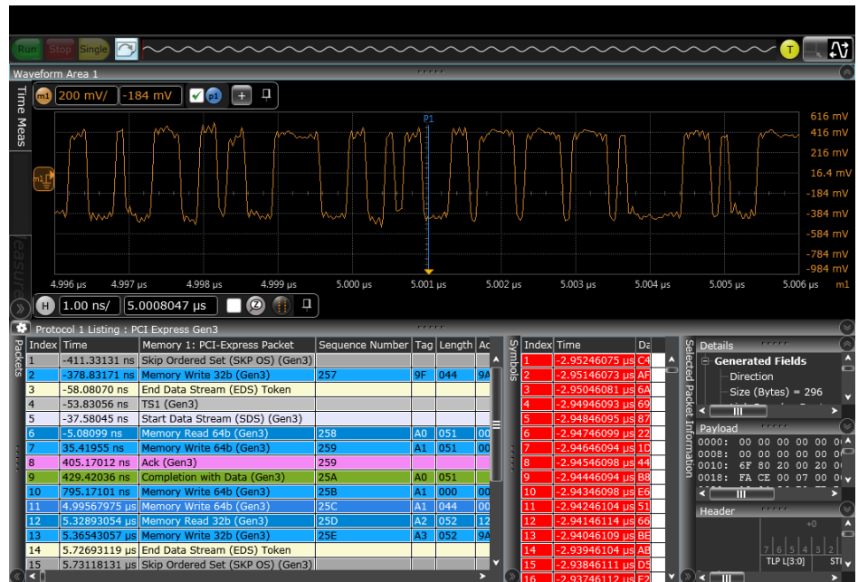
Z-Series decoding the PCI Express Gen3 packets.
