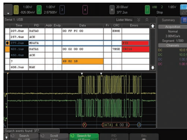
Figure 21. USB 2.0 trigger, decode and "lister" display.
