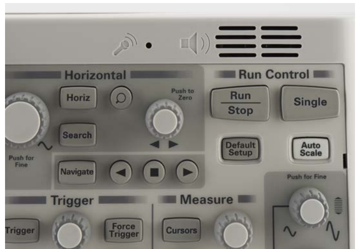
Figure 39. Voice control microphone and speaker.
