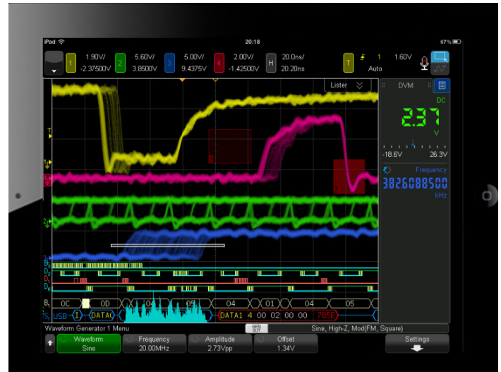
Figure 53. Controlling the 6000 X-Series via tablet device.
