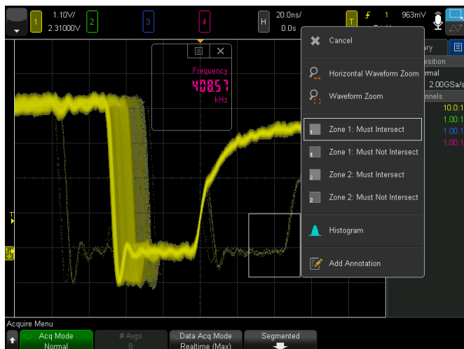
Figure 11. Draw a zone (box) around the anomaly.
