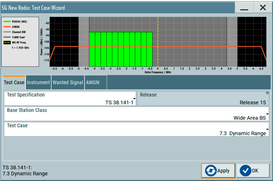
The 5G NR test case wizard allows the R&S®SMM100A to be conveniently and cleverly configured for BTS tests in line with 3GPP TS38.141
