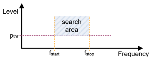
Figure 9-3: Basic principle of the signal search feature
