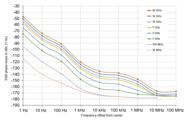
Typical phase noise sensitivity (start offset = 1 Hz, correlation factor = 1, signal level = 10 dBm)
