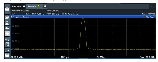
Figure 4-5: Calibration signal with optimized display settings
