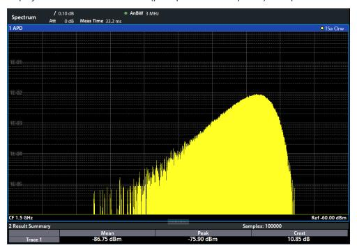
Figure 6-33: Amplitude probability distribution of white noise
