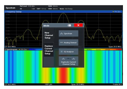
Figure 4-8: Adding a new measurement channel
