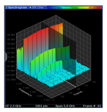
Figure 6-61: Three-dimensional spectrogram
