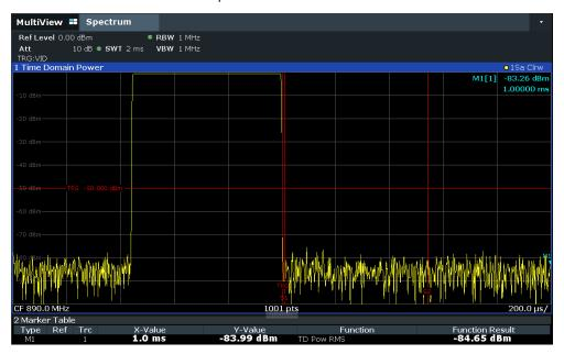
Figure 6-19: Measurement of the signal-to-noise ratio of a GSM burst signal in zero span
