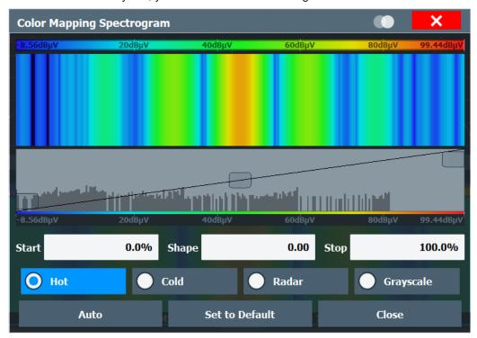
Figure 6-62: Spectrogram with (default) linear color curve shape = 0
