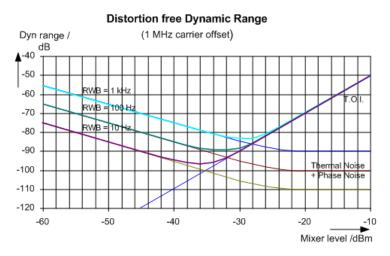
Figure 6-38: Intermodulation-free range as a function of level at the input mixer and the set resolution bandwidth
