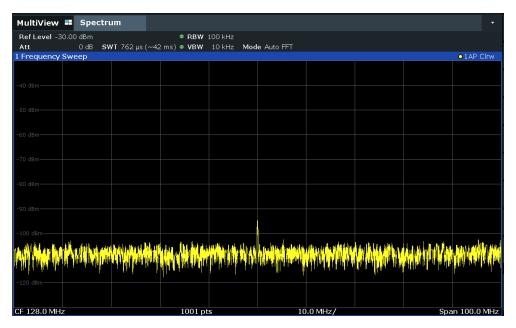
Figure 6-4: Reference signal at a smaller resolution bandwidth
