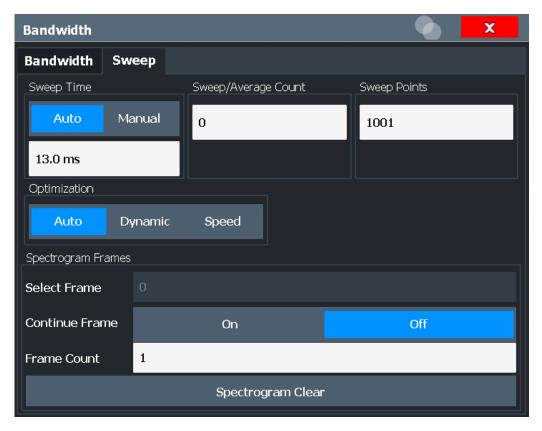
Figure 6-46: Sweep dialog box for spectrogram display
