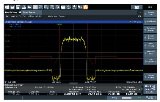
Figure 6-26: Detected peak display in SEM measurement
