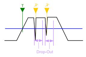
Figure 6-48: Effect of the trigger drop-out time
