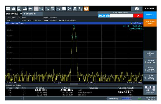
Figure 6-54: n dB down marker function
