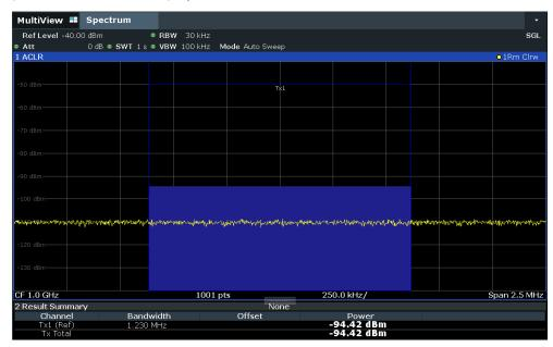
Figure 6-24: Measurement of the R&S FPL1000's intrinsic noise power in a 1.23 MHz channel bandwidth.
