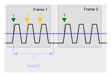
Figure 6-50: Effect of the trigger holdoff
