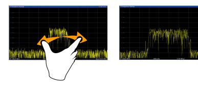
Figure 4-24: Spreading
