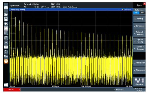
Figure 4-4: Calibration signal as RF input
