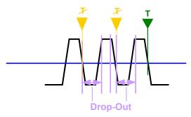
Figure 6-49: Trigger drop-out time for falling edge trigger
