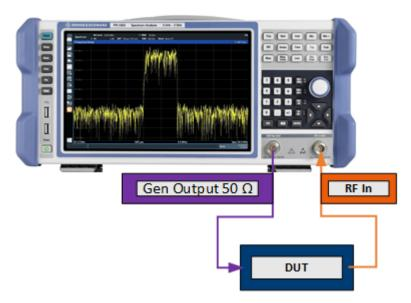
Figure 6-42: Test setup using the internal generator
