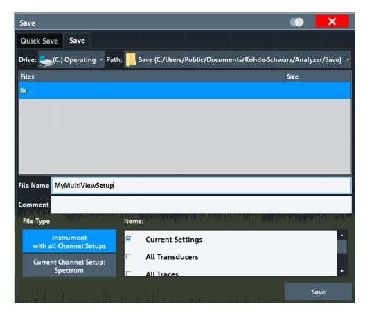
Figure 4-20: Saving the instrument settings to a file
