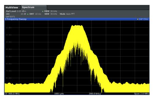
Figure 6-53: GSM signal with GATE ON
