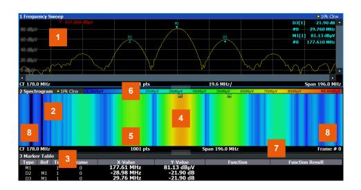
Figure 6-60: Screen layout of the spectrogram result display
