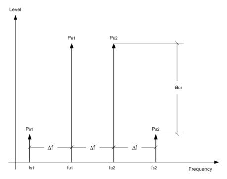
Figure 6-36: Intermodulation products Ps1 and Ps2
