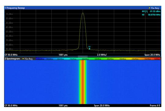
Figure 4-7: Spectrogram of the calibration signal
