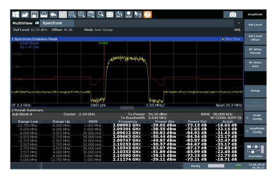
Figure 6-25: Spectrum Emission Mask result displays
