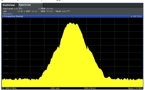
Figure 6-52: GSM signal with GATE OFF
