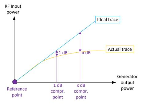
Figure 6-21: Compression point calculation
