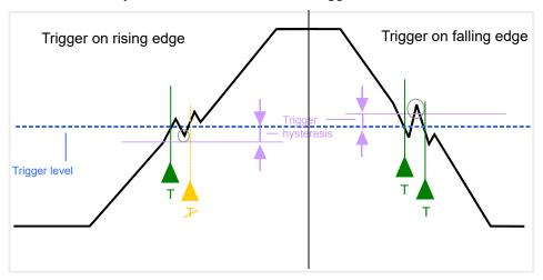
Figure 6-47: Effects of the trigger hysteresis
