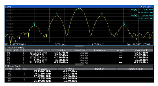
Figure 6-40: EMI measurement results
