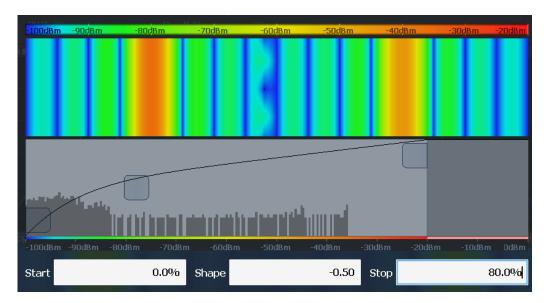
Figure 6-63: Spectrogram with non-linear color curve (shape = -0.5)
