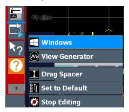
Figure 8-1: Inserting the Windows icon in the toolbar
