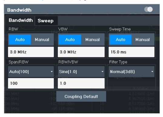
Figure 6-45: Bandwidth dialog box for RF measurements
