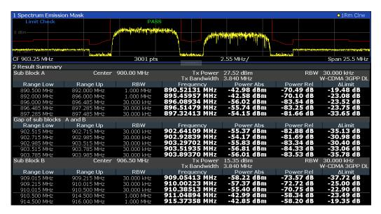
Figure 6-27: SEM results for multiple sub blocks
