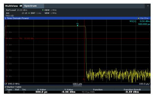
Figure 6-14: Measurement of the average power during the burst of a GSM signal
