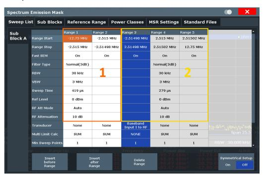
Figure 6-28: Sweep list using Fast SEM mode
