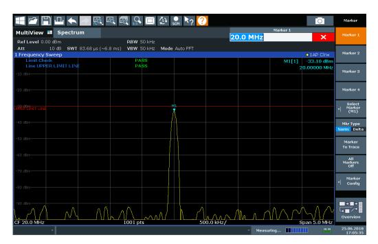
Figure 6-65: Example for an upper limit line
