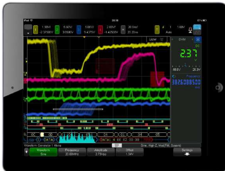
Figure 53. Controlling the 6000 X-Series via tablet device.
