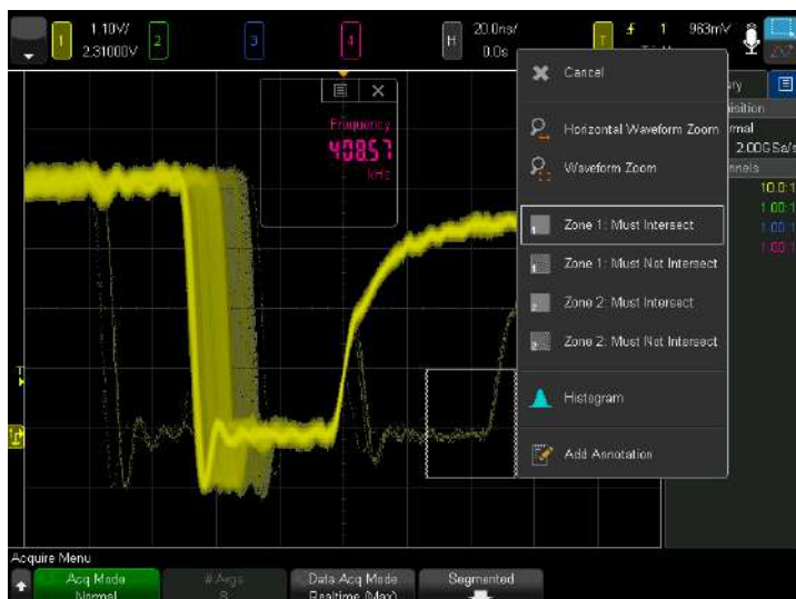
Figure 11. Draw a zone (box) around the anomaly.
