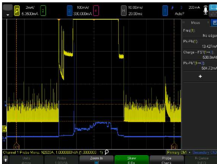
Figure 57. Capturing both zoom out and zoom in view of a cell phone's current consumption inside and outside of its sleep state.
