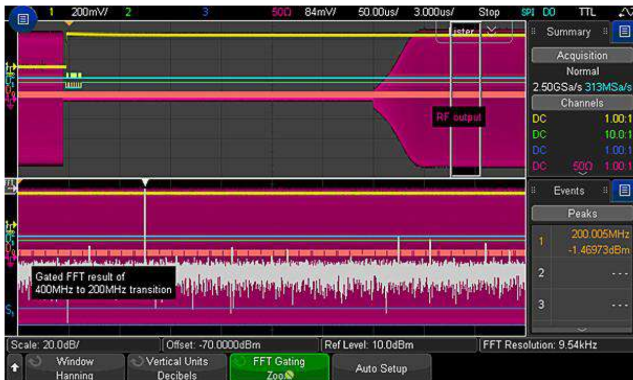
Figure 24. RF signal settled down at 200 MHz as indicated in the search list.
